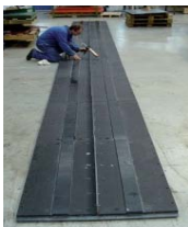
Bottom and side wall for chain conveyor
