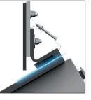
AirScrape is a newly patented German designed and manufactured conveyor belt skirting system which hovers freely above the conveyor belt, eliminating skirt friction & belt damage.
